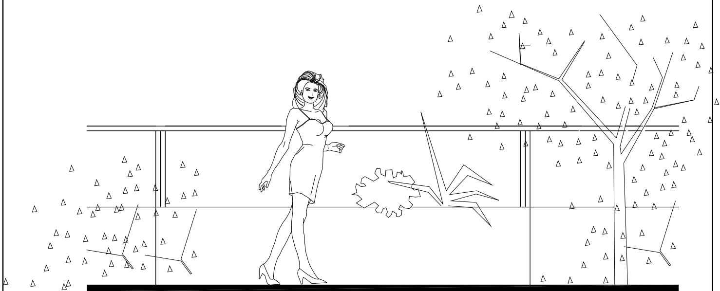
ELEVATION OF EXTERNAL FENCE FORMED WITH PANELS HORIZONTALLY PLACED
